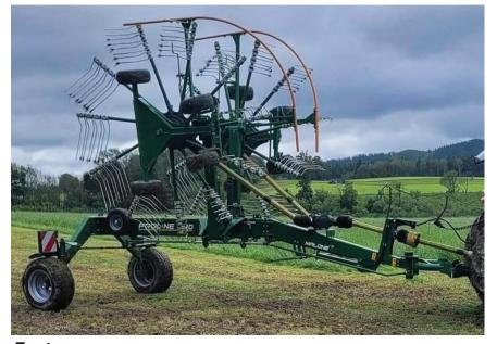
The Malone Proline 610 Rake is built exclusively for the intended use in the agriculture sector for the raking of common grass and cereal crops. The twin rotor rake follows the contours of the ground efficiently using the weight of the rotors on the ground and a single acting ram in the flotation position. The rake is fitted with a control box to allow the user to lift one side of the rake at a time. Making the job as efficient and easy as possible.
