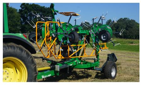
The Tedd-air 570T, 840T-U & Tedd-air 1120T-U is specially designed for forage tedding and spreading by means of rotating spring tines (double hook tines) attached to rotors.
